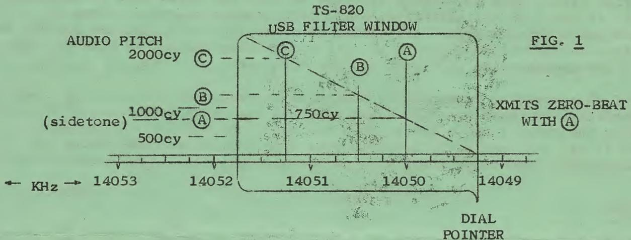
Now, let's suppose that (A) is a DX station, and he's working (B). You can zero-beat (B) (matching the sidetone pitch to signal (B)) by simply moving the tuning dial UP  $\frac{1}{2}$  KHz. This will cause pitch of (A) to drop to 250cycles, which is well within the receiver passband (window), as shown in FIG. 2.
